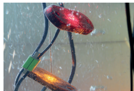
Test of leakproofness in a salt water column
